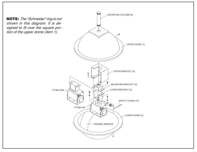
Figure 5. SS3000 Exploded Assembly Diagram
